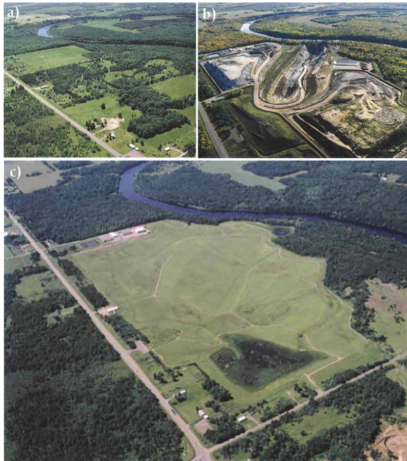
Flambeau Mine Site in the United States: a) before mining (1991), b) during mining (1996), and c) after mining (2002) 21 22
